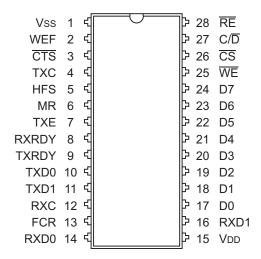
Pin numbers apply for plastic and ceramic DIP and for plastic PLCC. Consult factory for pin out of 48 lead ceramic leadless chip carrier.
